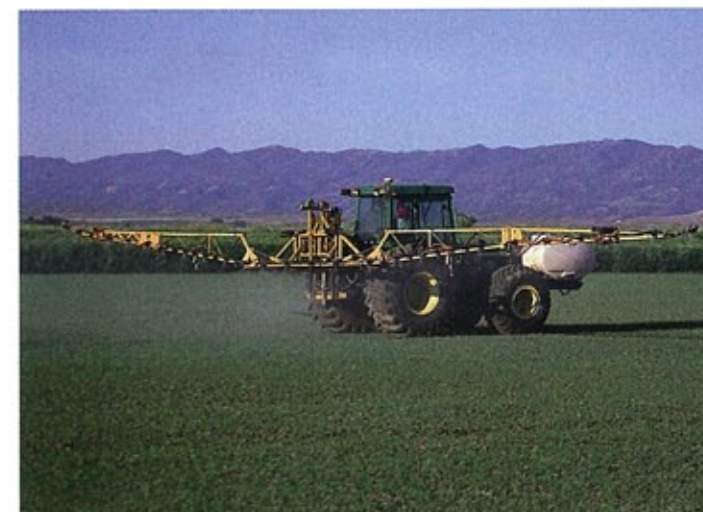
Different methods of herbicide application are used in California, including this ground rig with 30-inch wheels, above. The floatation tires mean minimal crop damage to rice. In addition to planes, Hiller helicopters, left, are also employed to make applications.
